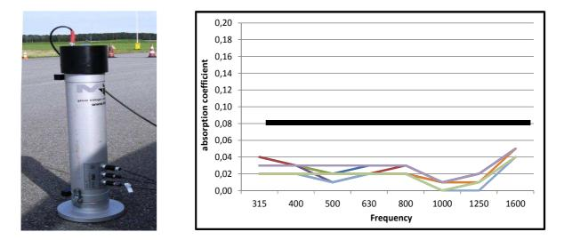
Fig. 8 – Left: picture of the impedance tube for in-situ measurements according to ISO 13472-2. Data processing is extended with respect to ISO 10534-2 by using three microphones and selecting the optimal pair based on the coherence function. Right: typical result for 4 different positions in the drive lane. The black line indicates the allowed maximum absorption.
