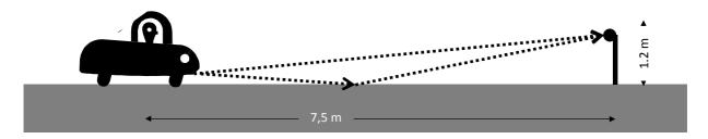
*Fig.* 4 – A simple ray tracing sketch of the propagation from the passing vehicle to the microphone. The reflection takes place in the propagation area.
