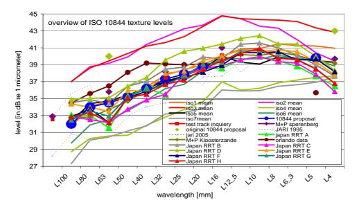
Fig. 2 – texture spectra of about 25 different test tracks in Europe and Japan. The blue dots represent the average value after removing the outliers. These averages define the reference wavelength spectrum for the ENDT calculation.
