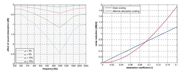
*Fig.3 –Left: effect of sound absorption vs. frequency for different absorption coefficients α, constant over frequency; it is clear that absorption works strongest in the 1 kHz frequency region. Right: effect of acoustic absorption on overall rolling noise level.*
