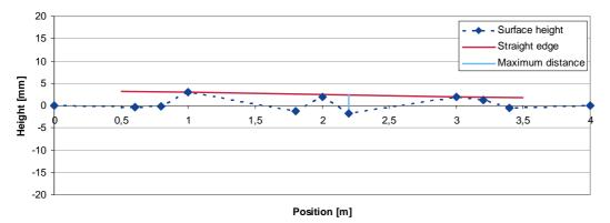
Fig. 9 - Example of a cross profile of a test track and a the positioning of the virtual 3 m beam on top of it. The light blue line segment indicates the maximum deviation.
