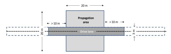
Fig. 1 – geometry of the test track according to ISO 120844:2011
