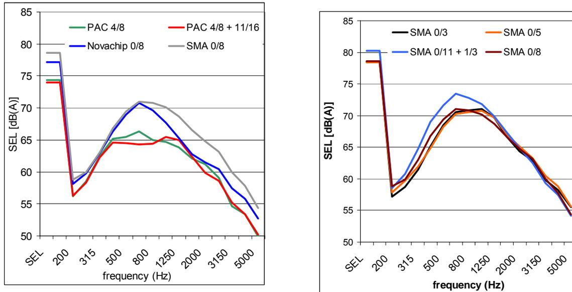
Figure 7 : 1/3 octave SEL spectra of composite vehicle (2S, 4D and 4T tyres), left: variation of acoustic absorption, right: variation of surface texture.
