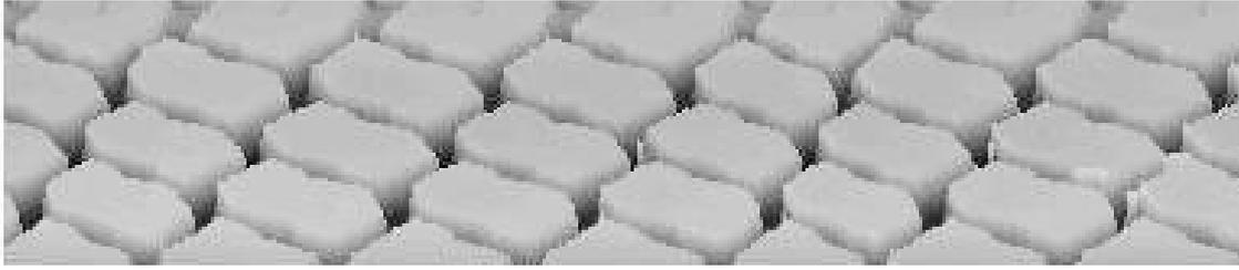
Figure 4: part of a scanned 3-dimensional tread profile of a tyre (shown is tyre Gd). Resolution of the scan is 1 mm in horizontal direction and 0.01 mm in vertical direction.
