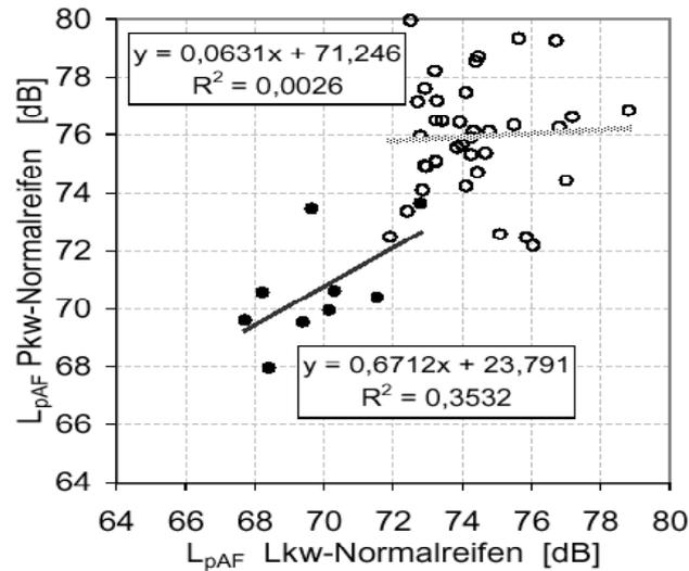
Figure 1: Relation between rolling noise of truck tyres (LKW-Normalreifen) and of passenger car tyres (“PKW-Normalreifen”) on several surface. Open dots are dense surfaces, solid dots porous surfaces [1].
