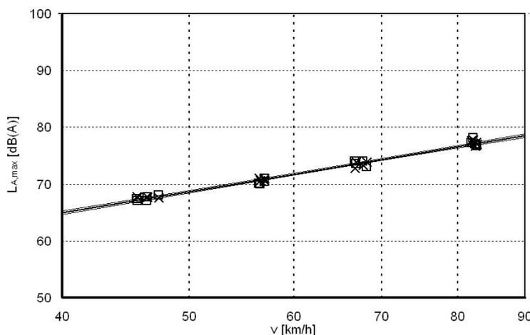
Figure 5: typical example of regression of  $L_{A,max}$  versus log of speed together with 95% confidence interval around regression line. Number of measurements: 36, level at 70 km/h:  $(74,3 \pm 0,2)$  dB(A), 95% confidence interval, slope: 38,6 dB/10-fold speed increment, residual error: 0,4 dB.
