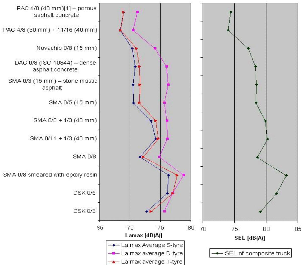
Figure 6: results of averaged levels of the tyres at 70 km/h at the test surfaces: left: rolling noise levels ( $L_{A,max}$ ) of the three types of HDV tyres at the test surfaces; right: total Sound Exposure Level of a vehicle, composed of two steering tyres, four traction tyres and four trailer tyres.
