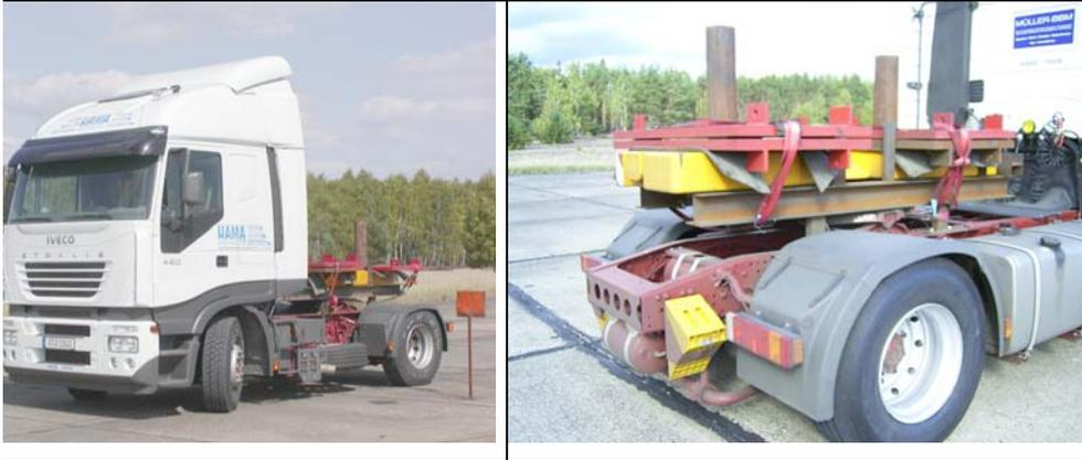
Figure 2: left: picture of test vehicle, right: extra weight mounted to meet the 70% tyre load requirement.
