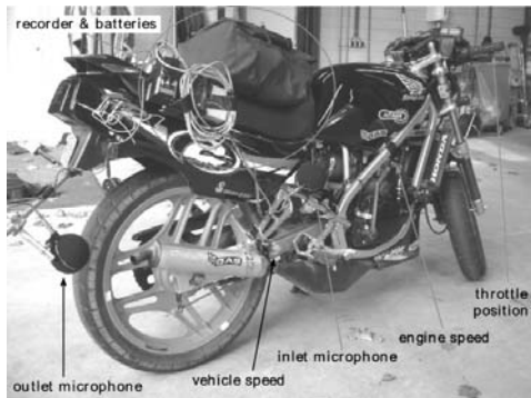
Figure 5: On-board noise measurement setup
