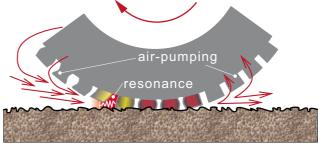
*Pipe resonance.* Each tread pattern, in contact with a rather smooth road surface, constitutes a system of pipe resonators. Their resonant frequencies depend on the geometrical properties but not on the rotation speed of the wheel.
