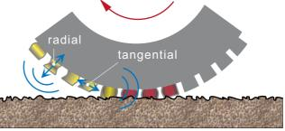
surface. The stick-slip mechanism is normally associated with situations where relatively high tangential forces are applied to the tyre (e.g. acceleration, breaking, cornering). The role of this mechanism for free rolling conditions is unclear.
