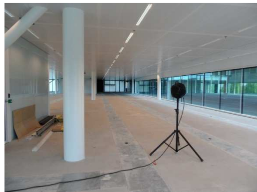
Figure 6a Measurement D_{L2,S} in existing building
