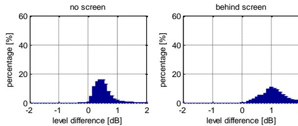
**Fig. 5.** Computed noise level difference for receivers for vertical position change of 1 m without and with noise screen in between track and receiver.
