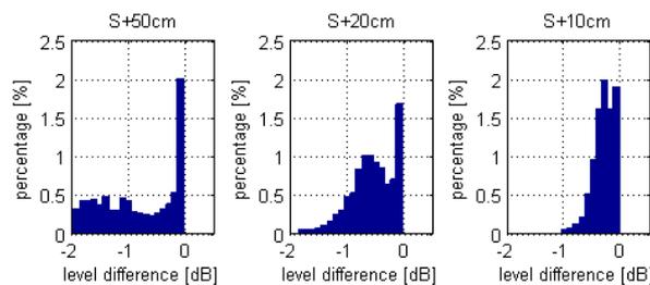
**Fig. 6.** Computed noise level difference with an increase of screen height of 50, 20 and 10 cm.
