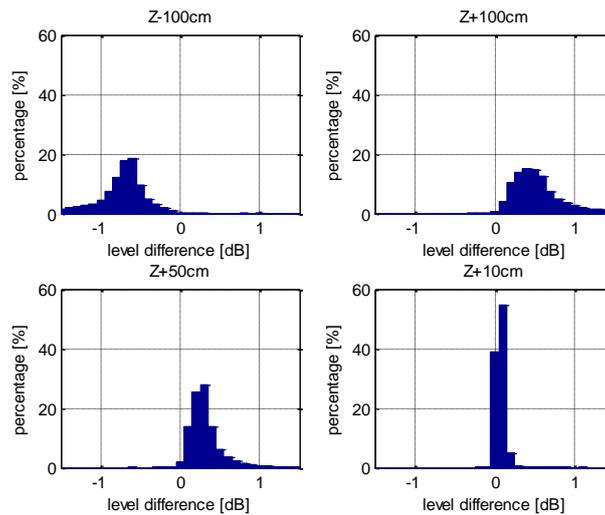
Fig. 4. Computed noise level difference for a vertical position change
