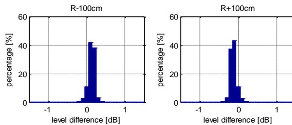
Fig. 2. Computed noise level difference for a distance change minus/plus 100 cm.
