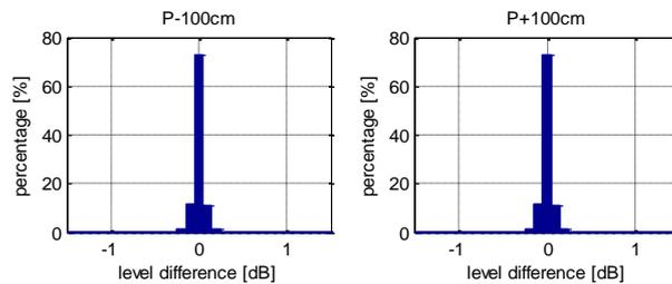
Fig. 3. Computed noise level difference for a parallel position change minus/plus 100 cm.
