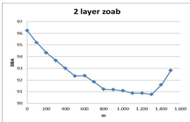
Fig. 3 - Variation of the CPX level over the length of test section 1.
