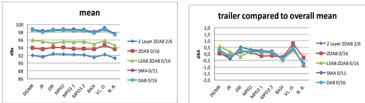
Fig. 5 - Left: averaged CPX levels of the 9 combinations over the 5 test sections. Right: deviation of the CPX level from each combination to the average value for that tyre section. Data for SRTT reference value at 80 km/h..
