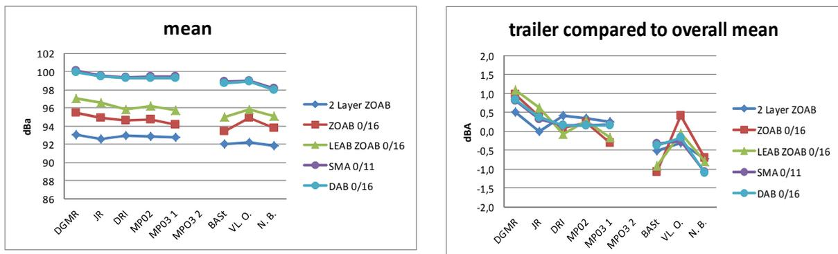
Fig. 4 - Left: CPX levels(average of left and right track) of the 9 combinations over the 5 test sections. Right: deviation of the CPX level from each combination to the average value for that test section. Data for SRTT tyre at 80 km/h.
