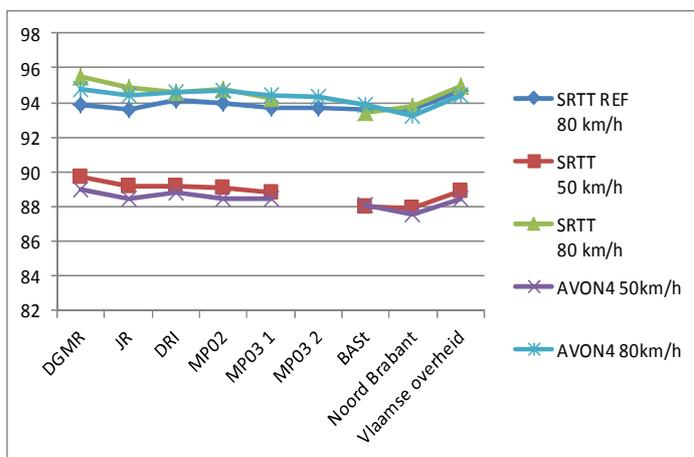
Fig. 6 - Results for all tyre/speed combinations on ZOAB 0/16 (n.b. the last two operators are interchanged compared to figure 4 and 5).
