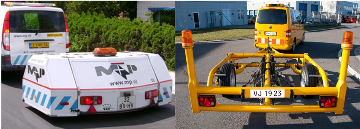
*Fig. 1 - Example of an enclosed and non-enclosed CPX system.*
