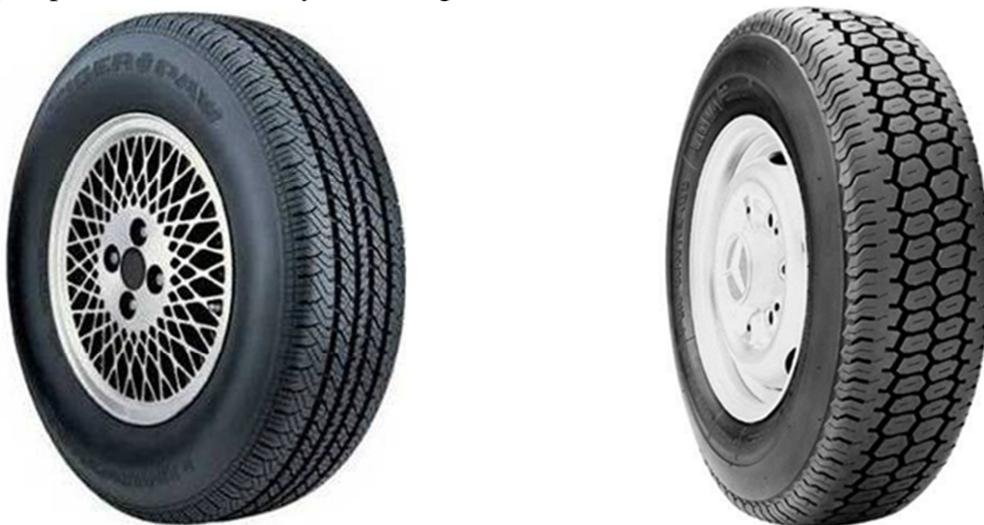
*Fig. 2 - Pictures of the two standard tyres used in the CPX Round Robin Test. Left: SRTT, Right: Avon AV4.*
