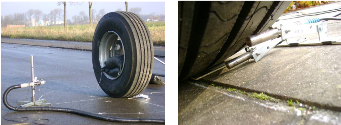
Figure 5 – Measurement set-up for determining the horn effect for truck tyres; left : noise source aimed at the tyre; right : microphones inside the tyre horn
