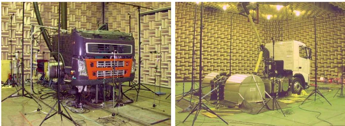
figure 8 – Volvo noise laboratory: the driveline rig (left) and the truck chamber (right)
