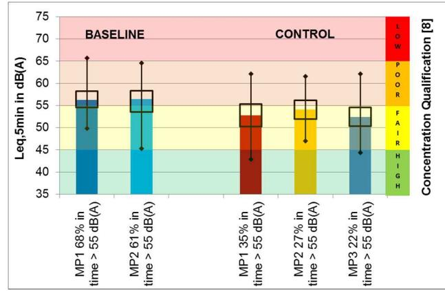
Fig. 5. results activity noise levels comparison baseline and control measurements (monitoring positions are given in fig 2 and 3).
