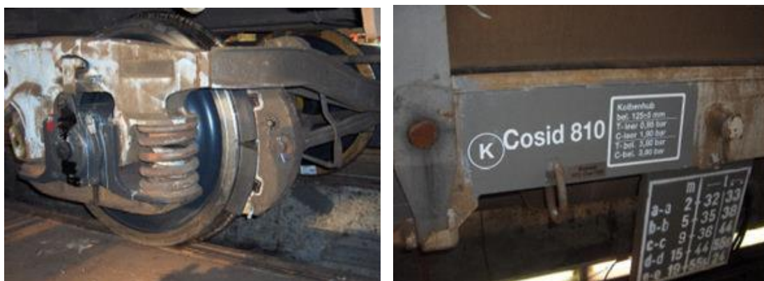
figure 8 Picture of a block brake with K blocks. Since K blocks imply modification of the braking system, (K) at the side of the train warns against wrong replacements (source SBB)
