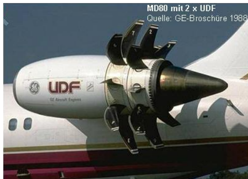
figure 31 Picture of a concept high efficiency engine design with counter rotating propellers.
