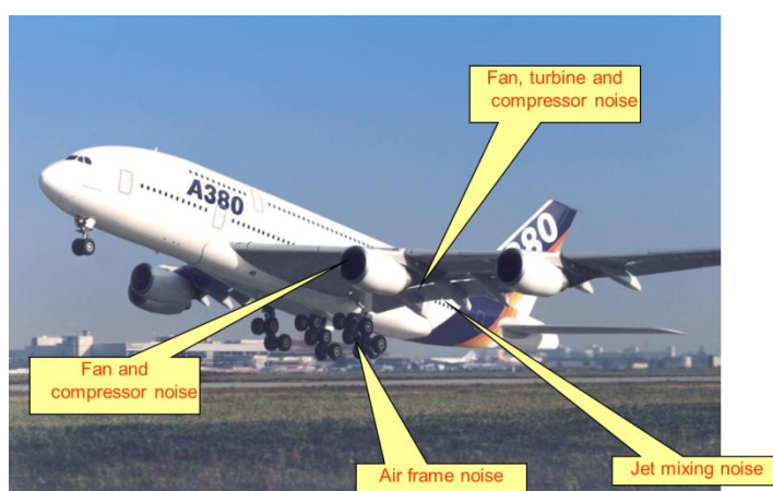
figure 6 Overview of the noise sources of a modern jet aircraft (see Chapter 14 for more information).
