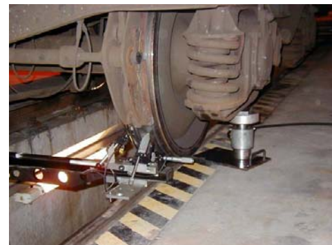
Figure 4: Direct wheel roughness measurement with a Müller-BBM RM1435 wheel roughness scanner
