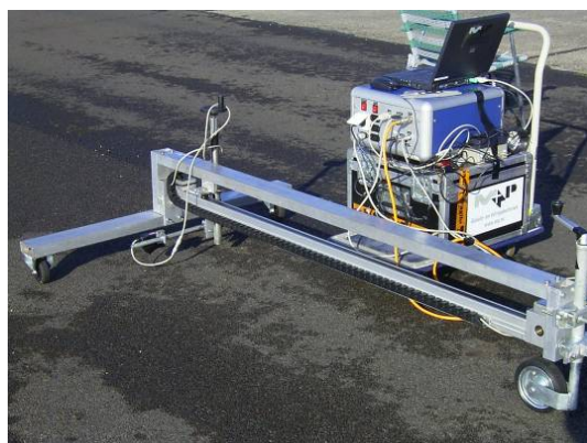
Figure 5: M+P static (3D) road surface roughness measurement system
