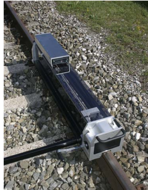
Figure 3: Direct rail roughness measurement with a Müller-BBM RM1200 rail roughness scanner
