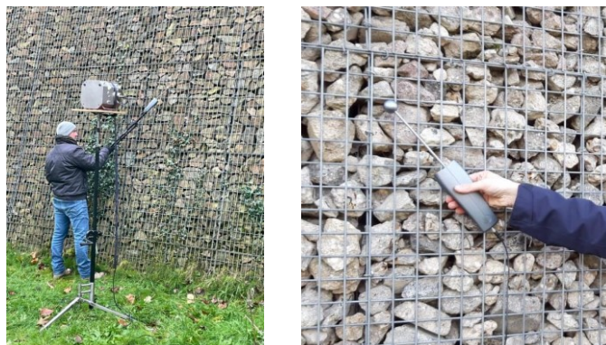
Figure 6: Performing scan or point measurements with the Sonocat instrument.
