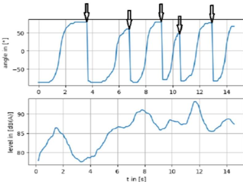
Figure 2: Diagram of a cluster of vehicles passing by. Upper diagram: Trajectory of the main noise source as function of the incidence angle. Lower diagram: sound pressure level of the passby
