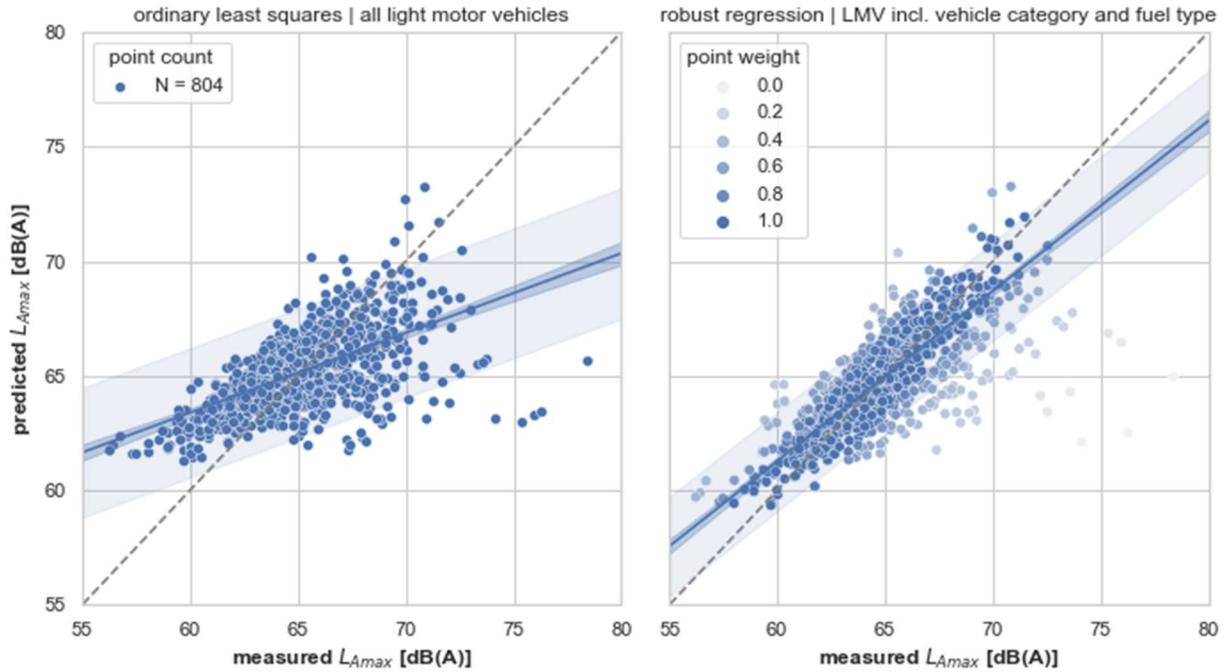
Figure 4: Predicted vs. measured  $L_{Amax}$  levels for light motor vehicles using different pre-processing models; left: ordinary least squares without vehicle info, right: robust regression with lower weights for outliers, with vehicle subcategory (M1/N1) and fuel type information. The blue line shows the linear regression through the points, with 95% confidence and prediction intervals
