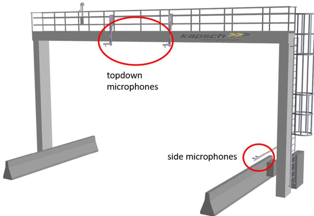
Figure 1:3D-model of the N-RSD measurement setup (*image provided by Kapsch TrafficCom AG*)
