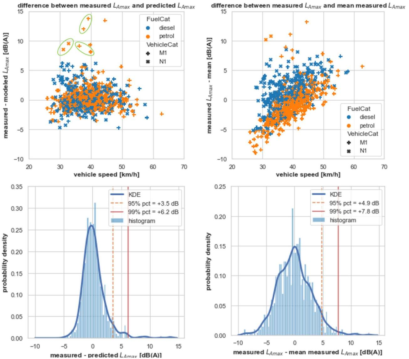
Figure 5: Distribution of  $L_{Amax}$  levels; left: measured minus predicted  $L_{Amax}$ , right: measured minus mean measured  $L_{Amax}$  (no pre-processing). Top graphs: difference values vs. speed, Bottom: distribution of differences as histogram and kernel density estimate (KDE).
