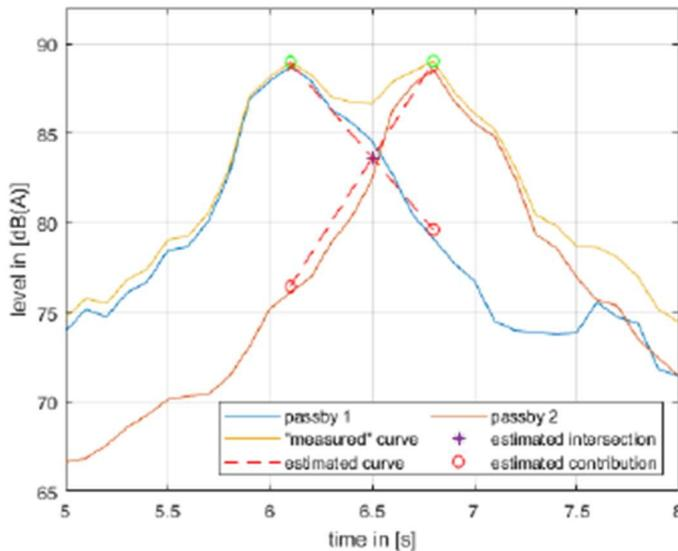
Figure 3: approach to estimate the contribution of every vehicle within the overall noise level.
