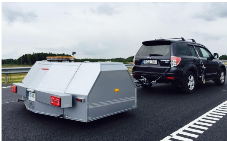
CoMeT CPX trailer with mobile laser texture measurement system FLASH|M delivered to Vilnius Gediminas Technical University in Lithuania
