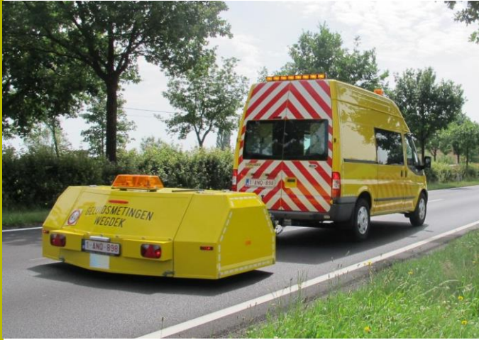
CoMeT CPX trailer delivered to the Flemish Public Roads Administration in Brussels, Belgium
