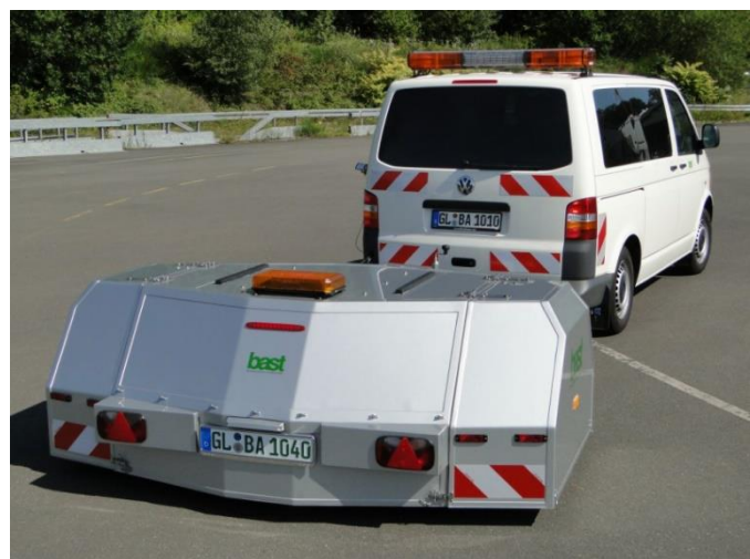
CoMeT CPX trailer delivered to Bundesanstalt für Straßenwesen (BASt) in Bergisch Gladbach, Germany. BASt is part of the German Public Roads Administration
