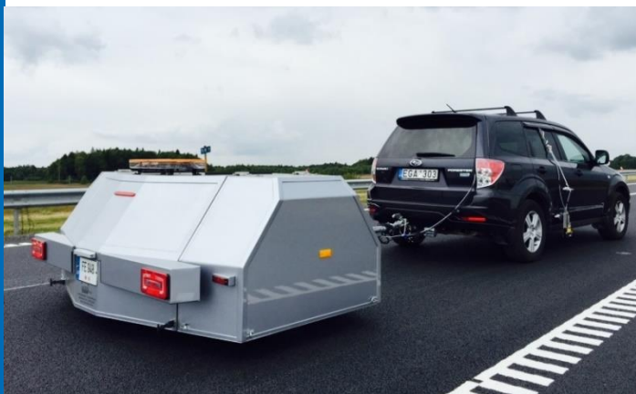
FLaSH|M texture system with CoMeT CPX-trailer in use by Vilnius Gediminas Technical University in Lithuania
