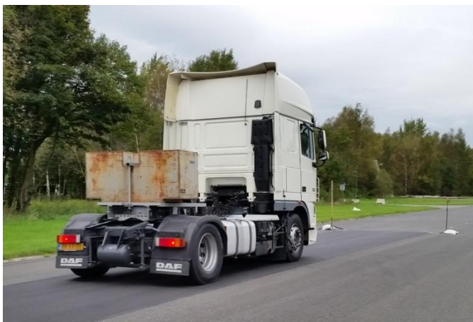
figure 4 Picture of the test vehicle and the extra load applied to meet axle load and vehicle load criteria in R117 [8].
