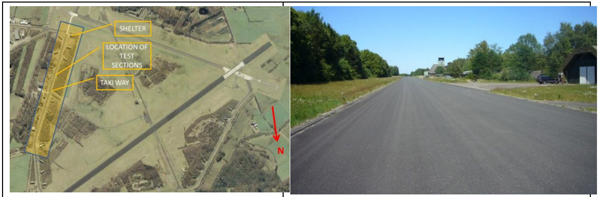
figure 1 Left: Aerial view of the test area with the test sections and the shelter. Right: Picture of the taxi way with the test sections. Picture is taken in NE direction.
