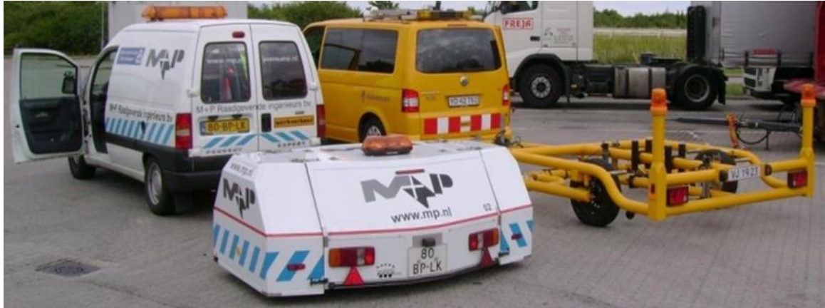
Figure 2 – Picture of two-wheeled versions of the CPX method, both covered and non-covered.
