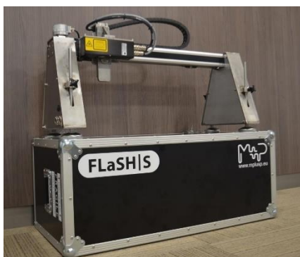
FLaSH|S texture system with profile length of 500 mm suitable for mounting in test stands
