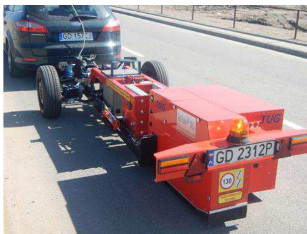
Figure 5: Example of a measurement trailer (TU Gdansk) for direct rolling resistance measurements
