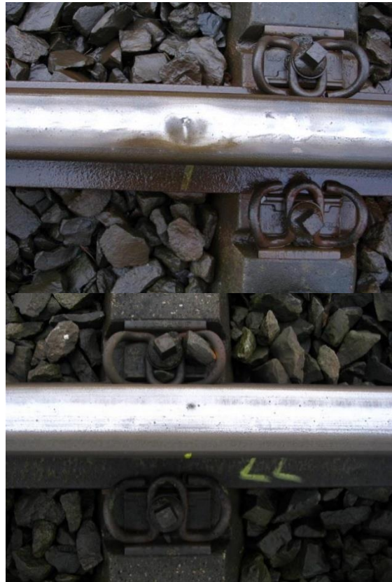
Type A (top) and type C (bottom) squat rail defects
