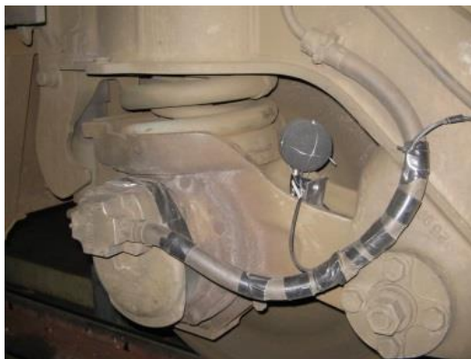
The ARRoW system mounted on a bogie of the Thalys high speed train.
