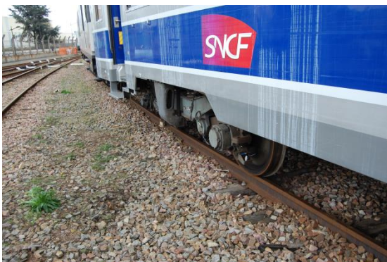
The ARRoW system mounted on the SNCF measurement train for the LECAV project.
