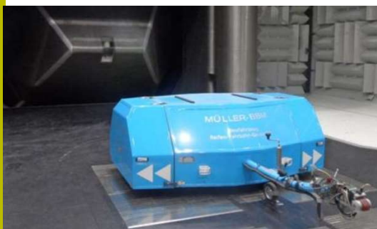
Wind tunnel testing of the CoMeT CPX-trailer
