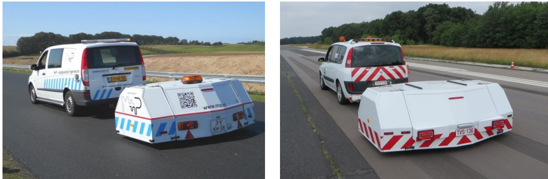
figure 8 CPX-trailer of M+P (left) and BRRC (right)
