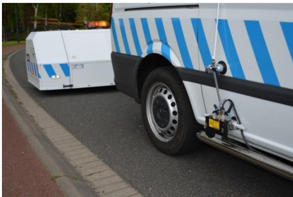
figure 22 Mobile laser texture meter used for height measurements of road markings
