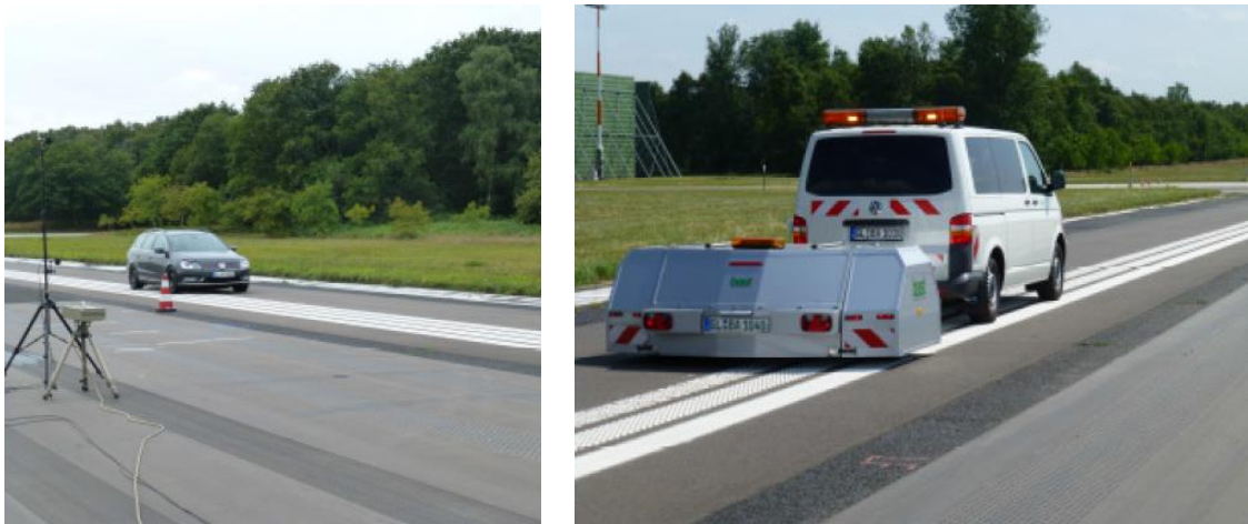
figure 1 Controlled Pass-By measurement (left) and Close Proximity measurement (right) [8]
