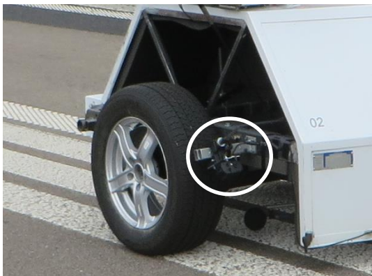
figure 9 CPX-trailer of M+P equipped with a camera system
